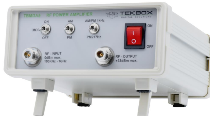
Picture 1 – TBMDA5 modulated wideband driver amplifier, front view
